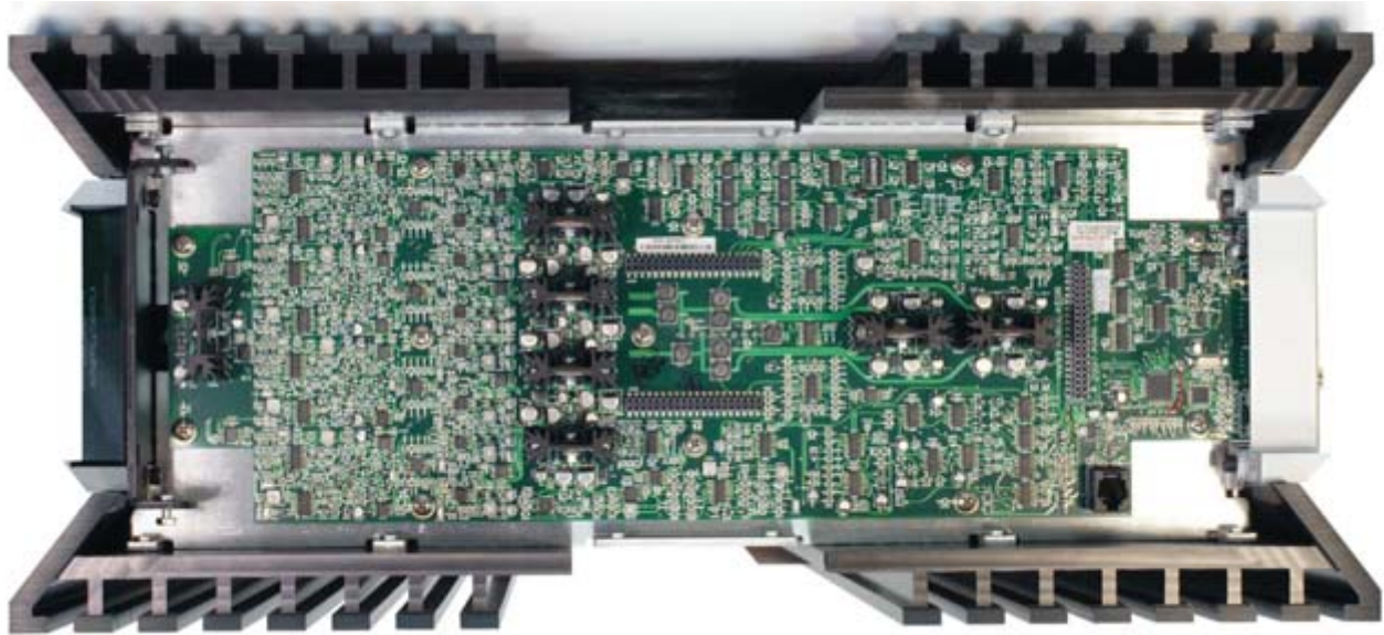
№53 Six layer modulator PCB contains about 1,500 parts
